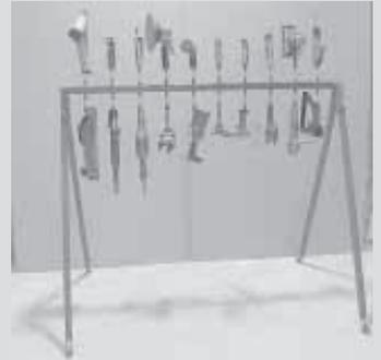
Metal stand mounts on 4 caster wheels. Horizontal top pipe comes with 20 quick couplers and space for 20 air tools.
