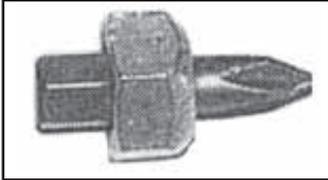
nut. I just slipped the nut onto the bit and used a wrench to turn it. Worked great. The idea would work on any type of drive bit."
