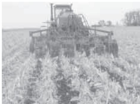
Rawson works closely with Brillion, which produces the Zone Commander deep tillage tool. This 6-row unit is deep tilling and placing dry fertilizer between rows of cornstalks.
