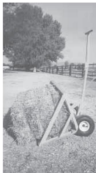
After lifting bale, cradle turns 90 degrees so you can push cart through narrow doorways or gates.
