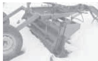
Rotor is chain-driven by a hydraulic motor. Rake is angled to windrow rocks to either side.
