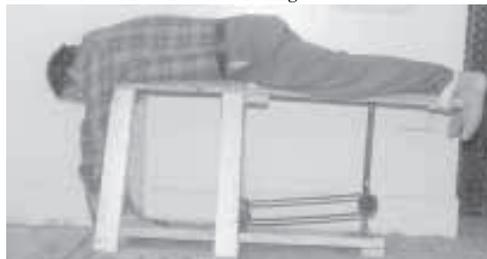
**A pitman crank on a sprocket, which is driven by an electric garage door opener, pushes hinged plywood sheet up and down. I doze off, my head stays upright."**
