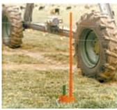
Pivot Post lets center pivot towers roll right over electric fence.
