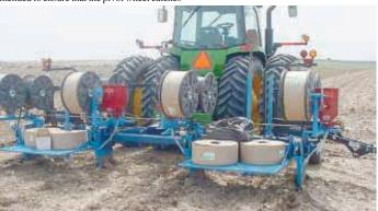
Harlan Downing equipped his tractors with the Trimble AgGPS Autopilot system. It lets him lay underground irrigation tape in precise rows.
