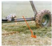
Once both pivot wheels have rolled over the wires, the post and fence spring back.
