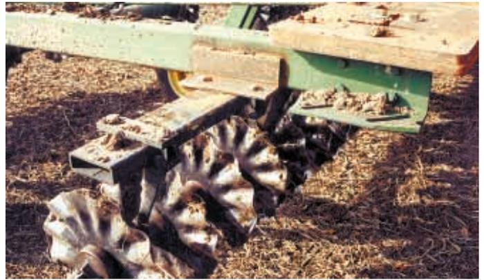
He replaced the original 22-in. dia. disk blades with 20-in. dia., 1 1/4-in. wavy coulters. He also added about 3,200 lbs. of weights to help the ripple coulters cut better.
