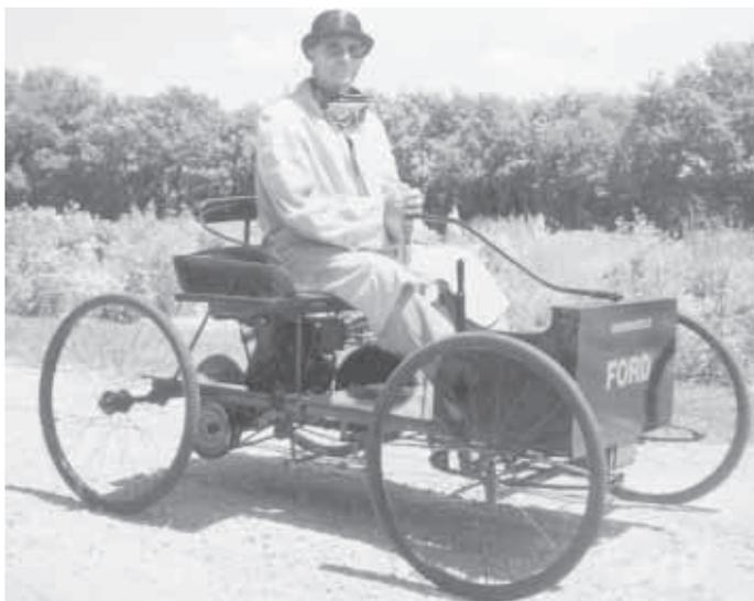
Allan Turner's replica "quadricycle" is built to the same width and length as Henry Ford's original. It's powered by a 7 hp engine off an old riding lawn mower.
