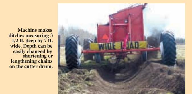
Machine makes ditches measuring 3 1/2 ft. deep by 7 ft. wide. Depth can be easily changed by shortening or lengthening chains on the cutter drum.
