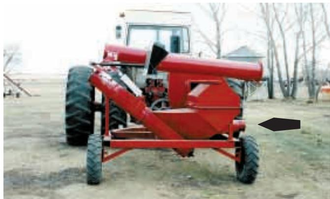
A 15-ft. long, 10-in. dia. transfer auger hydraulically folds out behind fan and delivers grain into a wagon or semi truck. Vacuum hose attaches to inlet pipe (see arrow).
