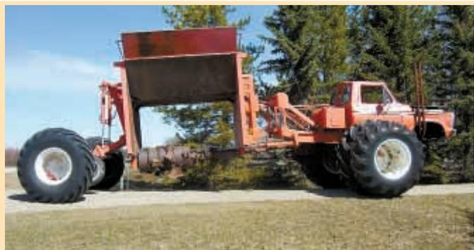
Cutter drum has heavy 1/2-in. decking chains with grader blades bolted onto outer ends.
