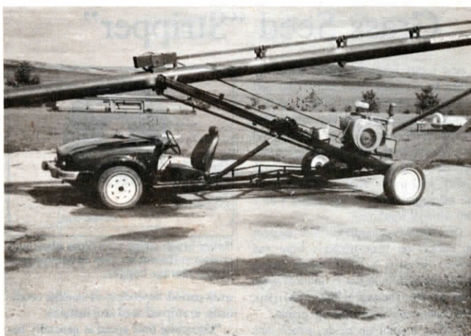
Ken Wise cut car chassis off behind driver's seat, then built a frame back to the auger.
