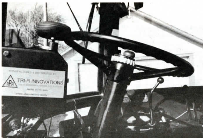
Small rubber-tired wheel rubs against steering wheel to automatically steer the tractor.
