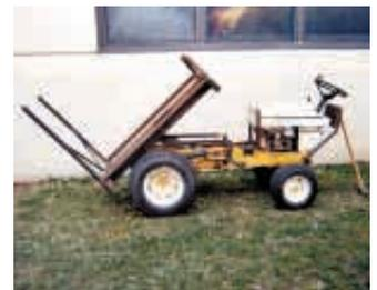
Dwayne Lowe turned a hydrostatic Cub Cadet into this walk-behind “mini forklift”. It has a 30 by 48-in. dump bed with forks on front that tilt down for loading.
