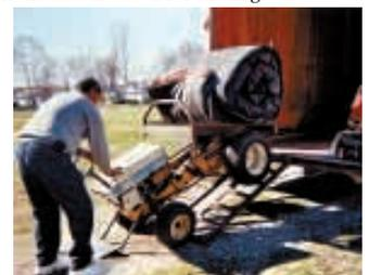
To operate the tractor, Lowe walks in front of machine and drives it backward. Operator can stand on fold-down front step to counter balance big loads.
