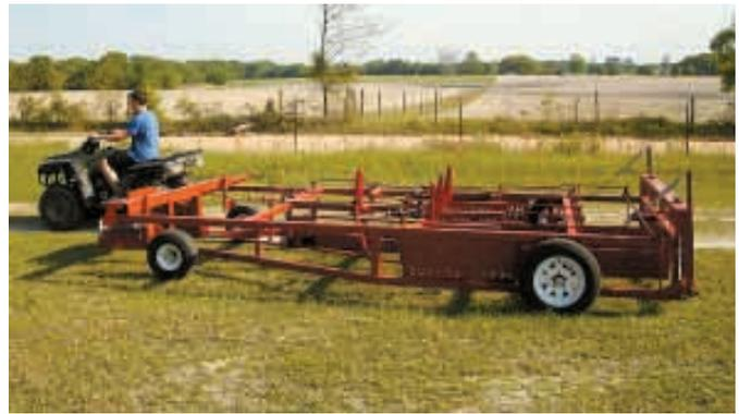
Lightweight, small square bale accumulator can be pulled behind an ATV, pickup, or small tractor.
