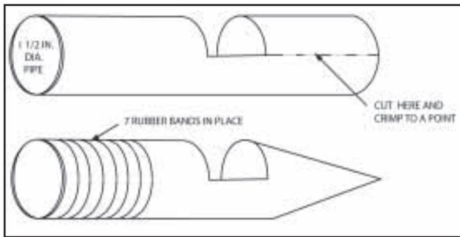
Baughman cuts pipe as shown (top), and bends the end to a point. To use, he slides pipe over scrotum and pulls tight with two fingers through hole in pipe before pushing off rubber band.
