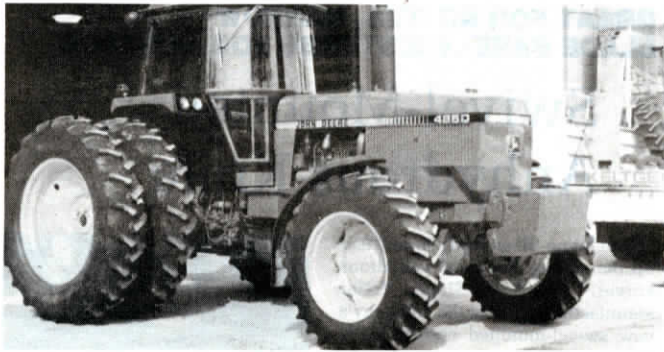
Dual "tall tires" equip bigger 2-WD tractors for the switch to narrow 22-in. rows.
