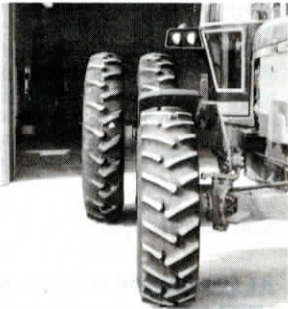
Tires raise tractor 5 in. to improve operation of 3-pt. equipment.
