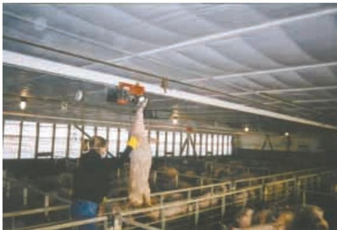
**Rail kit fits any building length and uses a wheeled trolley to carry the carcass. A hand-held control activates a 12-volt battery-operated hoist.**
