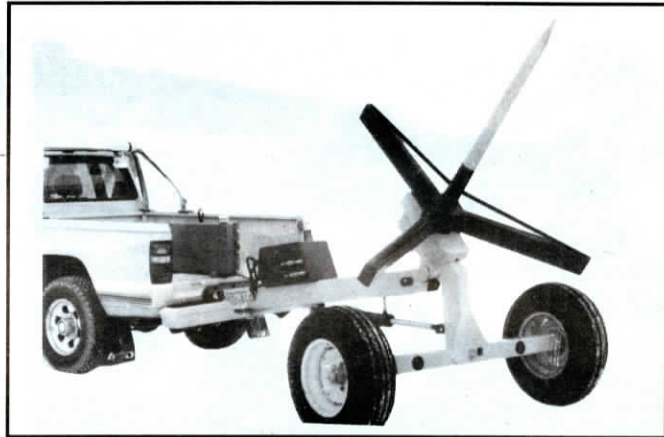
The "multi-use" bale-handling system consists of a 5-ft. long prong and 3-arm cradle.
