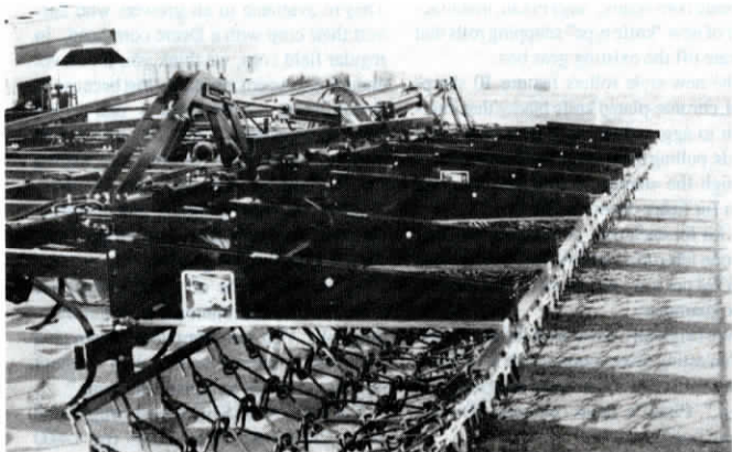
"Flex-Master" mounting brackets hinge to provide flexibility on uneven terrain.
