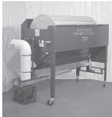
**Roto-Fingers Pea-Bean Sheller operates on 120 volts and shells up to one bushel in 3 to 10 min.**
