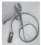
Auxiliary grounding device uses a pair of vise grips, allowing you to hold small parts in the desired position while completing the grounding circuit.
