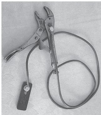
**Auxiliary grounding device uses a pair of vise grips, allowing you to hold small parts in the desired position while completing the grounding circuit.**
