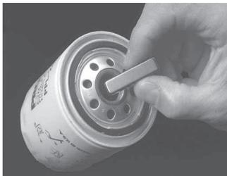
**Magnet catches metal fragments too small for an oil filter to stop. It's designed to be dropped into the center hole of any spin-on oil filter with a metal core.**
