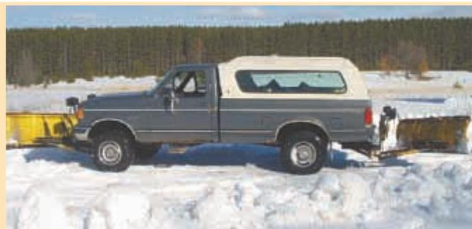
"It lets me plow snow in both directions so I never have to turn the truck around. That reduces my plowing time by half and also saves on fuel," says Alan Strange.
