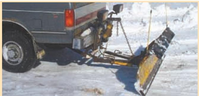
Strange made his own mounting kit for the plow. It's operated by a self-contained battery and hydraulic pump that mount in the pickup bed.
