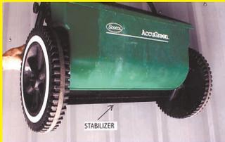
plying Gorilla glue to all mating surfaces, I installed a 3/4 by 2-in. stabilizing board by using a rubber mallet to tap it in place. A tarp strap placed around the hopper held it tight while the glue dried overnight. A little black paint and it looks like factory material. Now the spreader does a nice, even job. (Lee de Vries, 43251 Rodgers Mountain Loop, Scio, Oregon 97374 ph 503 394-3088)
