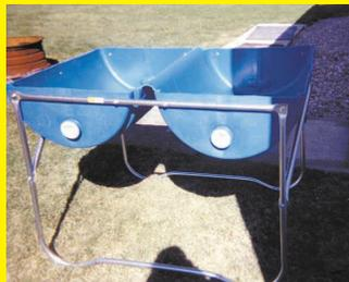
I made a roomy double wash tub that's easy to clean out by cutting a 55-gal. drum in half lengthwise. I left it connected on one side and bent it back, mounting the two half-barrel tubs on a stand made out of metal conduit. The tubs are easy to clean off by unscrewing the caps at one end. **(Richard Faber, Tiffin, Ohio)**
