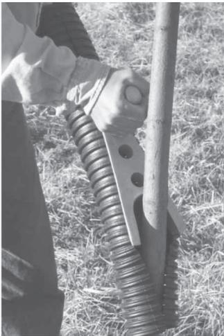
Wide end of tool spreads tube apart, making it easier to slide tube around tree trunk.
