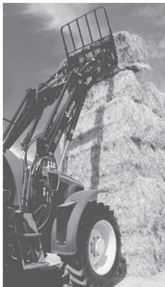
Loader’s parallel linkage provides up to 15 ft. of stacking and dumping height, which the company says is equivalent to most compact telescoping loaders.
