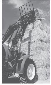
oader's parallel linkage provides up to 15 ft. of stacking and dumping height, which the company says is equivalent to most compact telescoping loaders.
