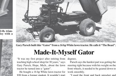
some tender loving care," he says. Parsch stripped off the mower deck and sheet metal parts and used the rear rack from a 4-wheeler to support the steering wheel. He moved the gas tank and battery and added linkage, allowing easy access to the hydrostatic transmission lever. Parsch also switched the foot brake into a hand lever. "It can be locked in case I want to get off the machine
