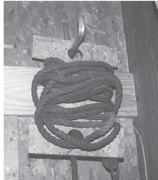
**Dan Neuman, Loami, Ill.:** You don't have to be a navy boatswain's mate to get neat control of your ropes, says Dan. He uses 15 by 12-in. sections of plywood to make this quickie rope storage system. Both sides of the plywood are notched to make it look like a big letter "T". Then he drills a hole into both the top and bottom of the plywood, making it easy to hang it on the wall.
