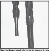
large drill bits with a Morse taper (right) to an R-8 shank.
