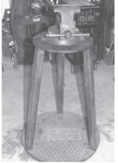
surplus store. The manhole cover is heavy which makes it stable and it's round, so it's easy to roll around our shop. We used existing holes in the manhole cover to attach the vice's three legs. Works great."
