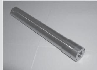
New, thicker stainless steel rod has a bronze nut that fits into the motor.
