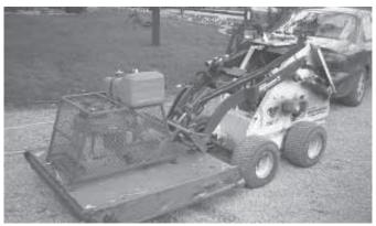
Kyle Herring mounted a trailing mower on front of the machine by using a mini skid mounting plate. He also replaced its small motor with a 15 hp twin cylinder. A brush guard protects it.
