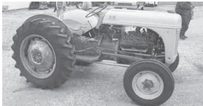
Kit costs \$995 and contains all the hardware needed to connect the V-8 engine and clutch assembly to the Ford 8N transmission and frame. Knasel says it takes about 8 to 10 hours to install.
