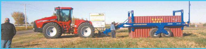
Dory Container Traveler will revolutionize how farmers transfer grain from the field to the end user, says inventor Dory Tuvim. The idea is to move shipping containers full of grain, instead of transfering grain from combine to wagon to bin to truck, etc.
