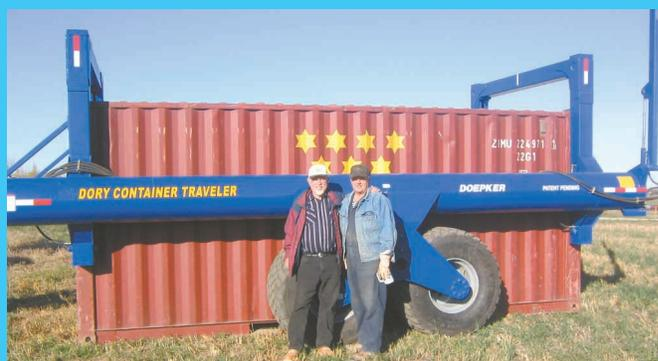
**Dory Container Traveler consists of a pair of horseshoe-shaped frame members attached to a subframe on wheels. It hauls containers that hold up to 1,100 bu. of grain.**
