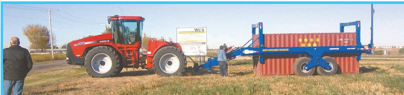
**Dory Container Traveler will revolutionize how farmers transfer grain from the field to the end user, says inventor Dory Tuvim. The idea is to move shipping containers full of grain, instead of transferring grain from combine to wagon to bin to truck, etc.**
