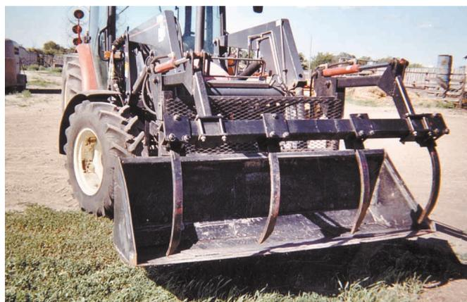
**Grapple fork has four 2-ft. long curved shanks spaced 2 ft. apart. Each shank measures 1 in. thick by 2 in. wide.**
