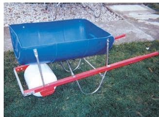
Faber cut a 55-gal. plastic drum in half to make wheelbarrow bucket and used a 20-lb. propane tank for the wheel.
