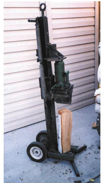
Portable wood splitter was made out of scrap metal and an 8-ton bottle jack, which powers the splitter.
