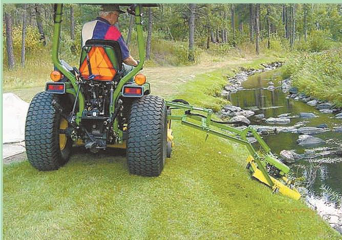
Push mower can be extended as far as 4 ft. out to the side of tractor.
