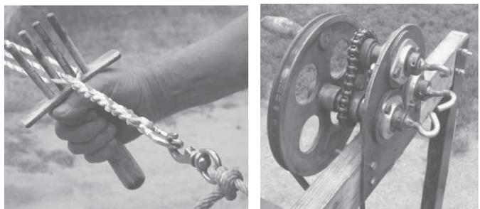
Four-pronged divider (left) is used to keep twisting strands apart. Strands attach to hooks welded to the end of each shaft (right).
