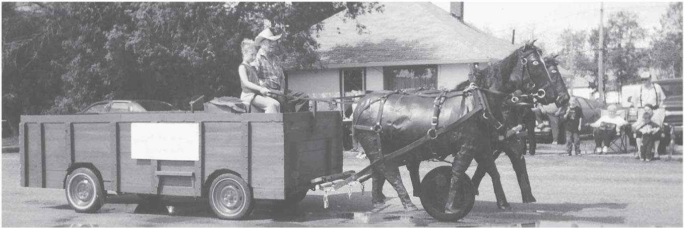
Self-propelled wagon is made from a 1975 Datsun station wagon with steering wheel and controls on front of the wagon box. Horses look real from a distance.
