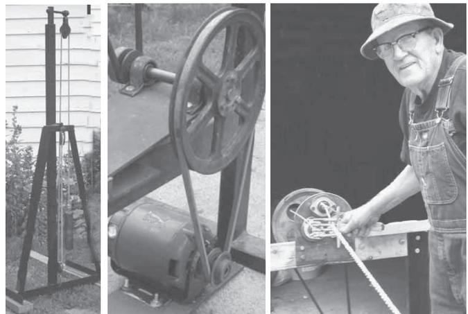
Rope maker consists of a 33-in. high, triangle-shaped metal stand with three pulleys that support a weight block (left). Rope leads from it to another metal stand with an electric motor at the bottom and the rope-making unit at the top (center). Pearson uses divider to twist three strands of rope together into one (right).
