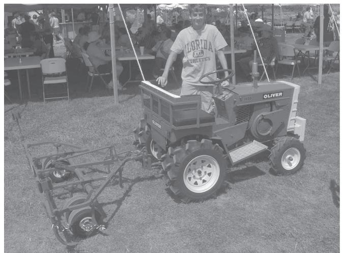
Swanson painted the orange and white Jacobson tractor Oliver green with white wheel rims. It has dual lugged tires on back and lugged single tires on front with a floorboard on each side. He replaced the original seat with a 36-in. wide one that holds two people.
