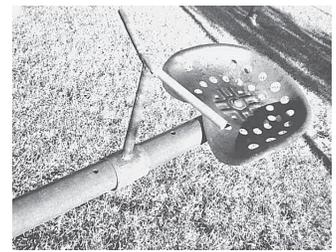
A 12-in. length of the axle sticks up out of the 36-in. dia. wheel's hub (left). Homemade handlebars at the end of the pipe are welded to an adjustable sleeve (right).
