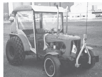
This modified Allis Chalmers goes 40 mph because Marion Klutzke took off its reduction gears and replaced the wheels with the front end off a 1959 Buick car. He added a pre-1940 Chevy truck 4-speed transmission to provide slow speeds.
