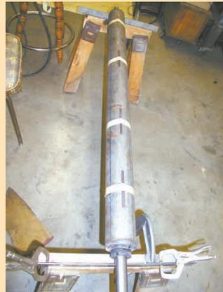
Flighting mounts on a 1.25 in. dia. steel shaft fitted with a 4-in. dia. center pipe. Gerken balanced it as he went along with small pieces of steel stock.
