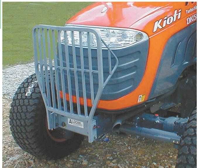
Bolt-on guard is designed to fit specific tractor brands.
