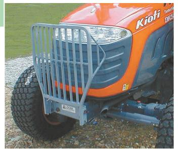
Bolt-on guard is designed to fit specific tractor brands.
