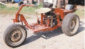
The "Little Red Horse", as Collins calls it, is powered by a 5 hp Briggs & Stratton engine and has the 4-speed transmission off a Volkswagen Rabbit.
