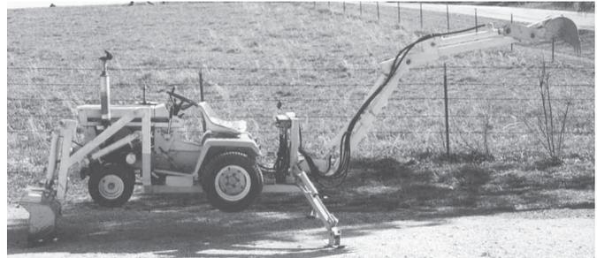
**Loader is made from 1 by 2-in. heavy wall rectangular tubing. Its bucket measures 38 in. wide and is made from 3/16-in. thick steel plate. Backhoe bucket measures 8 1/2 in. wide and is tilted up or down by a 3 1/2-in. dia. cylinder.**
