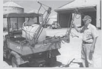
Sprayer's 10-ft. boom is equipped with four 30-in. long drop nozzles. The wings fold up manually for transport.
