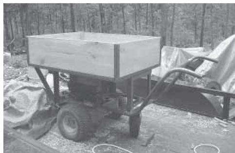
Lester Rose used the engine, transmission and gearbox out of an old riding mower to make this motorized dump cart.
