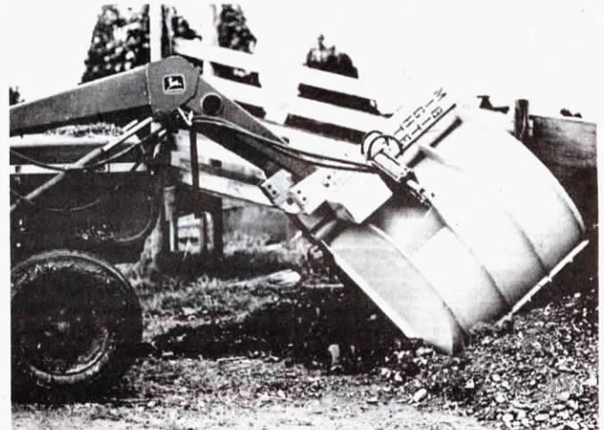
Jaws on the Mighty Bite close up tight to pick up 1,500 to 1,800 lb. bite without spilling.
