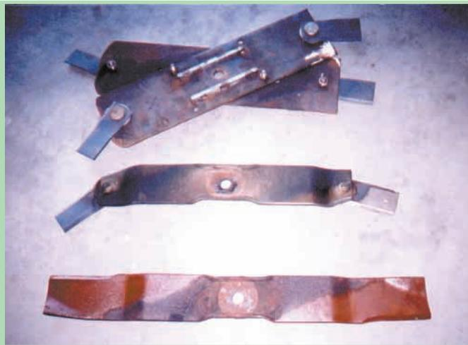
**Top blade is an experimental one while bottom blade is an original untouched blade. Gallaher says the simplest arrangement - the middle blade - works best.**
