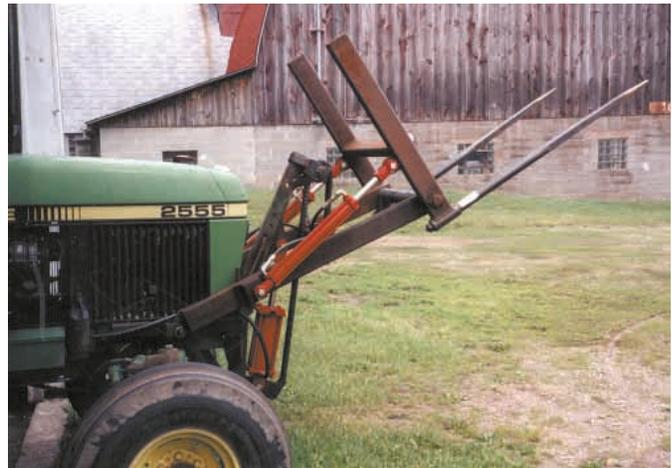
**Built from square tubing with a pair of commercial bale spears on it, loader can lift 1-ton bales up to 5 ft. high. "It's quite a bit lighter in weight than a commercial front-end loader," Dan Krueger points out.**
