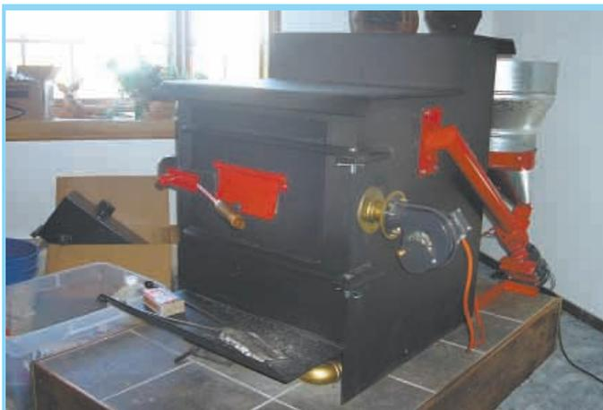
Leihgeber's stove burns wood, coal, corn, used motor oil, cooking oil, stove pellets, wood chips and other materials.
