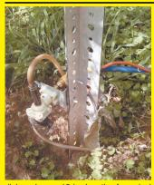
dishwasher, a 12-in. length of surgical tubing, and a short length of aluminum angle iron on which all components are mounted. The valve attaches to a bracket that's screwed to the angle iron. The extension cord runs up to the time clock and opens the valve to let air out of the surgical tubing, which then flaps back and forth
