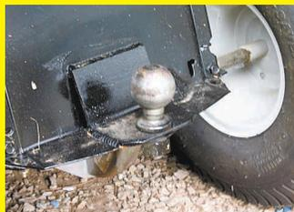
I didn't want to use my big tractors to pull small wagons and trailers around the yard so I made a hitch for my riding mower by bending a small 90 degree "L" out of steel and welding it to the back of the mower. Then I just put a ball hitch on it. It works really well. **(Ken Allison, Mansfield, Ark.)**
